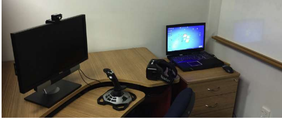
Figure 6. Experiment components including monitor, joystick, HMD, laptop, and HMD tracker placed at the top of the screen [23].
